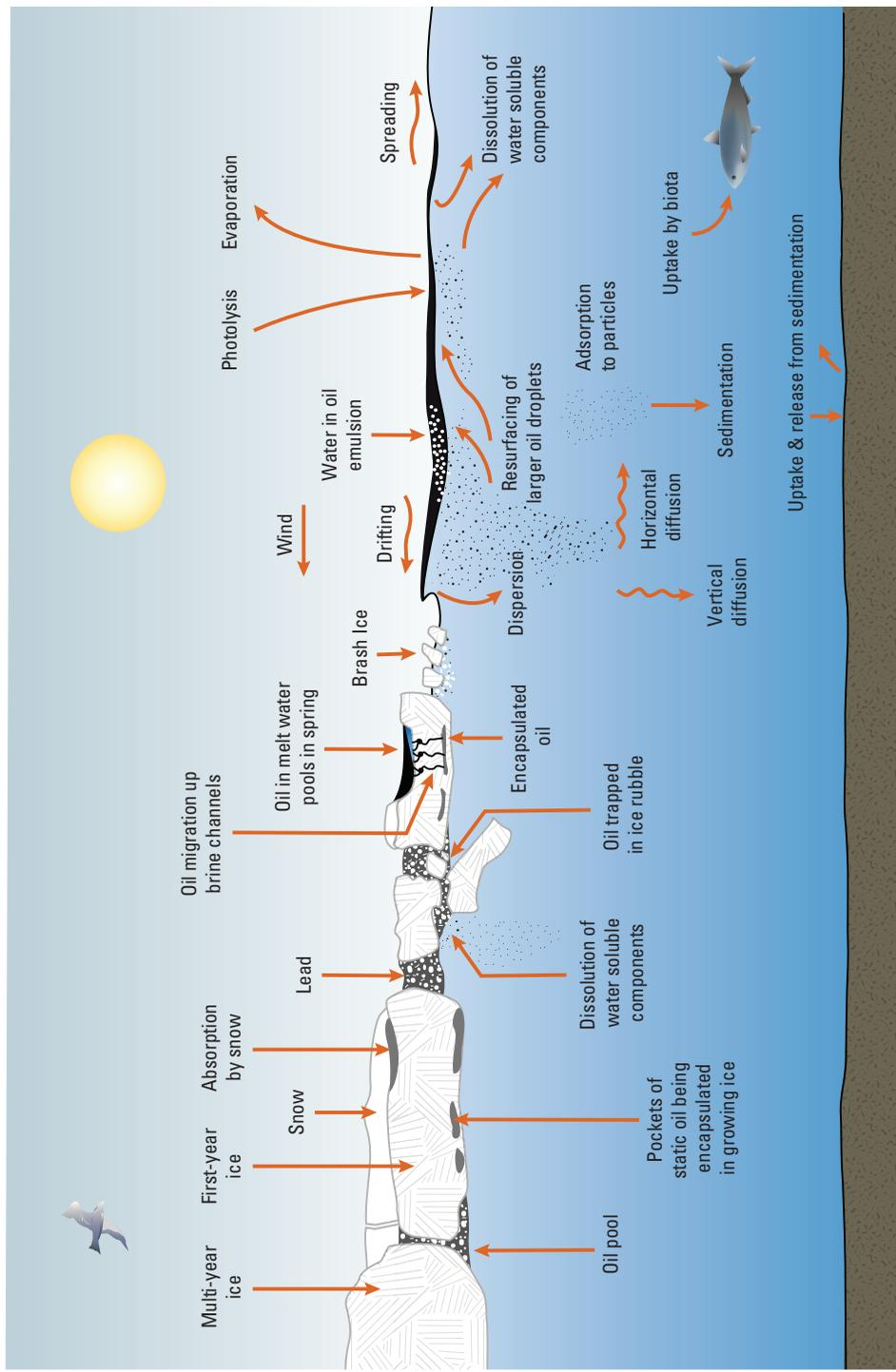
**Figure 3.2** Environmental processes that affect oil behavior and weathering in open water and in ice. SOURCE: Modified from Daling et al. (1990) and A. Allen.
