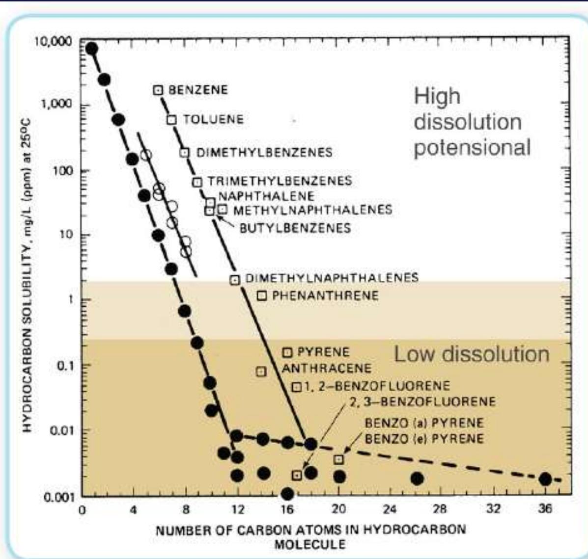
**Figure 6: Solubility per carbon number for hydrocarbon molecules, (Modified from McAuliffe, 1987 IOSG - proc. Pp 275-288)**
