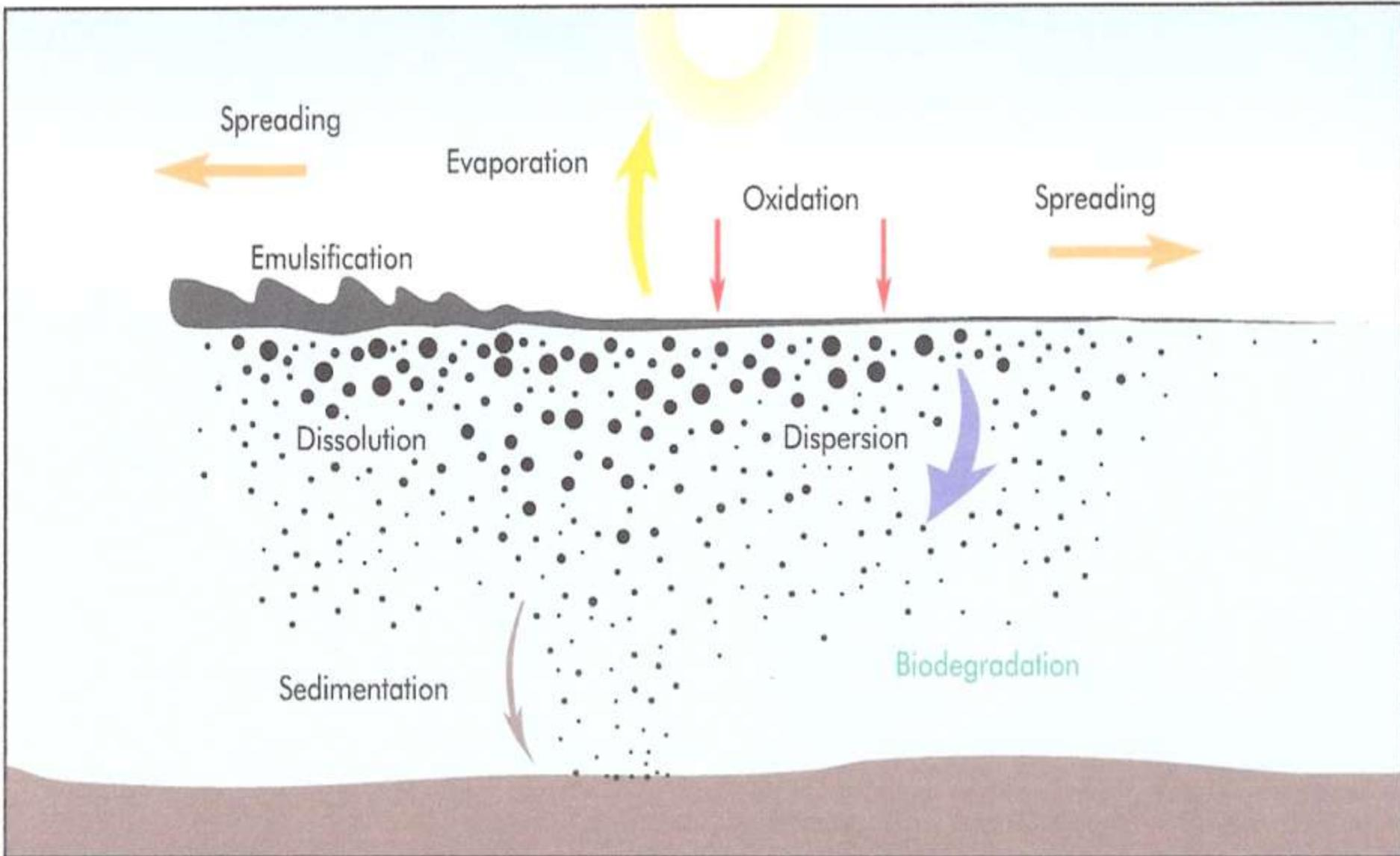
Figure 3: Processes acting on spilled oil.
