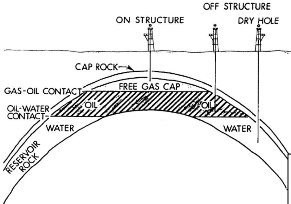
Fig. 11-5 Details of a saturated pool
