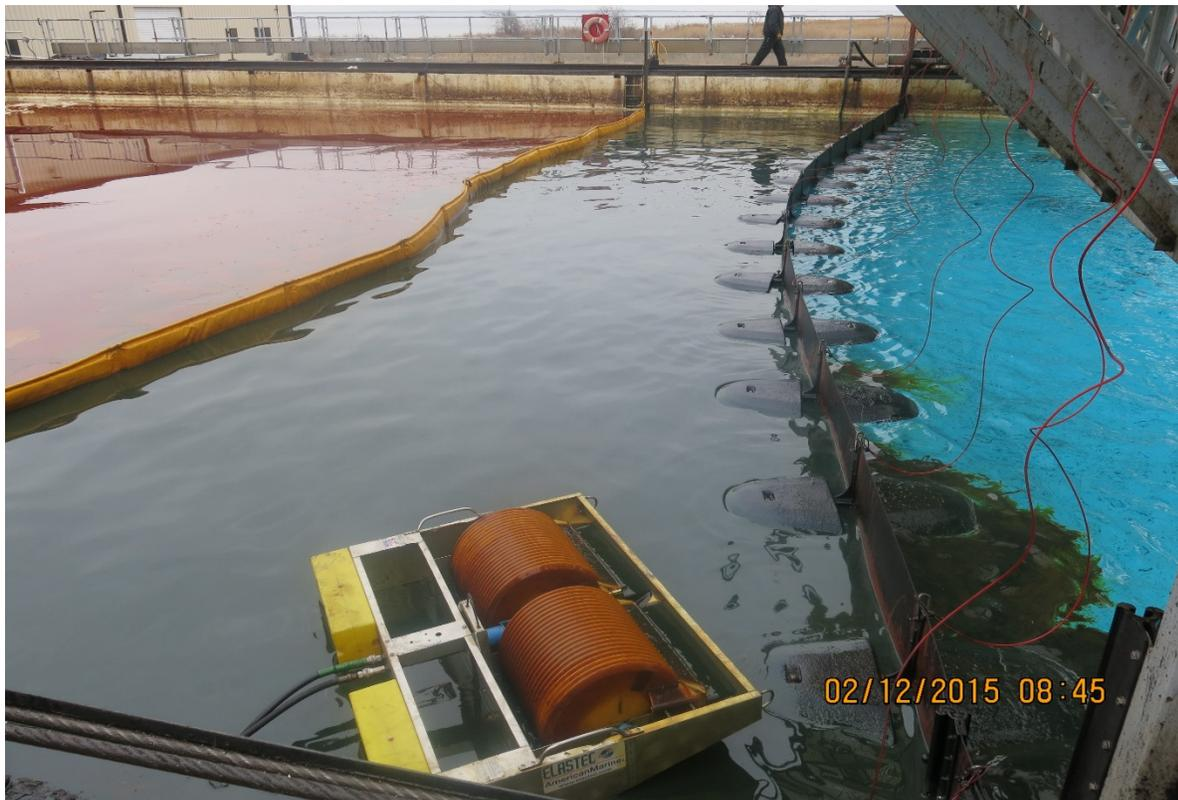
Figure 2 Oleophilic skimmer recovering oil after weathering period.
