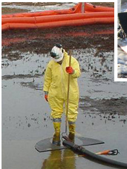
Figure 36. Manta ray skimmer in use and close-up view (inset)
