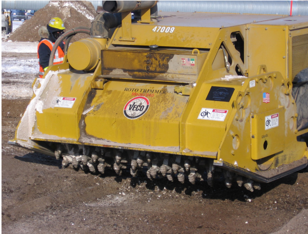
Figure 65. Trimmer excavating contaminated soil
