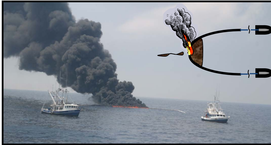
Figure 9407-6: Boats pulling fire boom in a U-configuration (DWH Spill – 2010)
