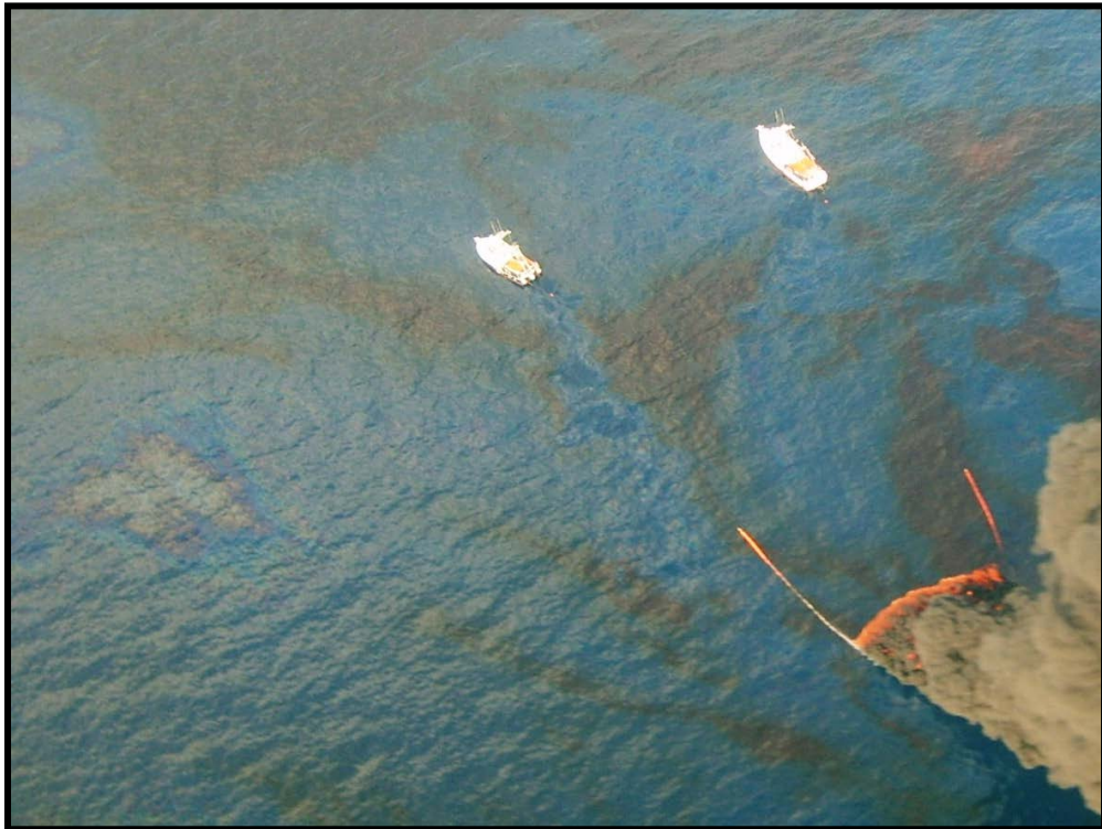
Figure 9407-9: Safe and efficient feeding of low-volatility oil to an ongoing burn (DWH, 2010).
