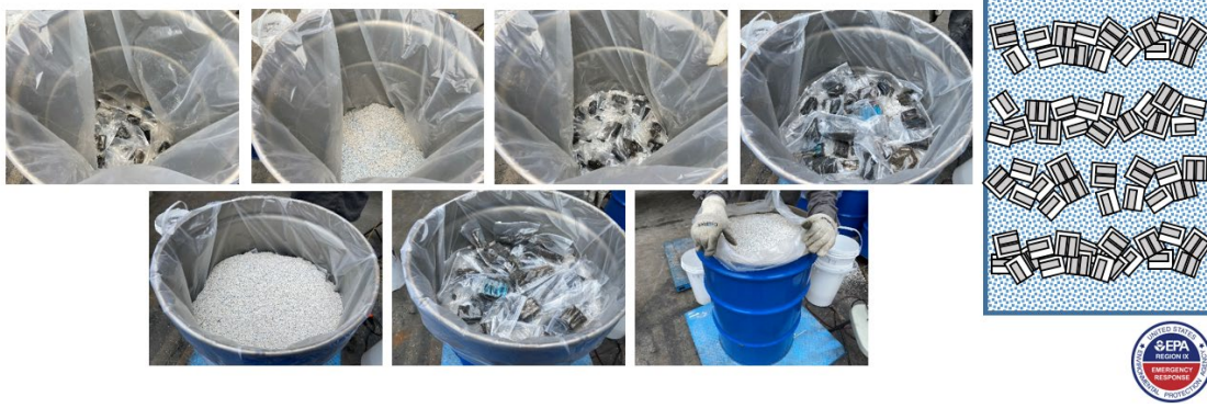
Figure 9: Small lithium-ion batteries can be transported according to Department of Transportation (DOT) Special Permit-16532 in a regular drum with cell block packing materials.
