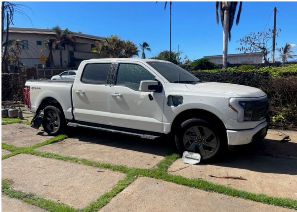
Ford F150 Lightning with visible heat damage. Taillights melted, wheel wells melted, discoloration of paint, plastic trim melted. Nearby structure fire.
