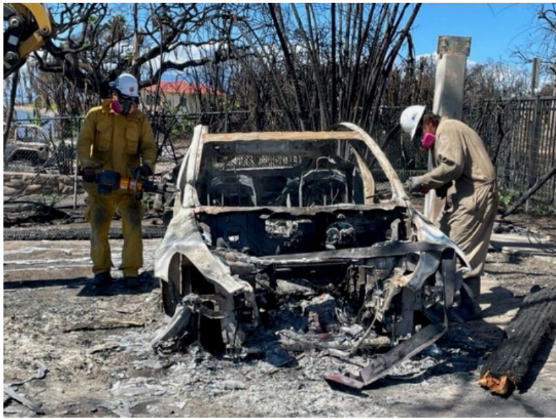
(Left) Rescue spreader and cutter. (Right) Cutting roofing support beams (A, B, C pillars) prior to flipping vehicle for battery pack access on some vehicles.
