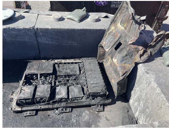
Figure 6: Nissan Leaf electric vehicle with prismatic battery cell technology.
