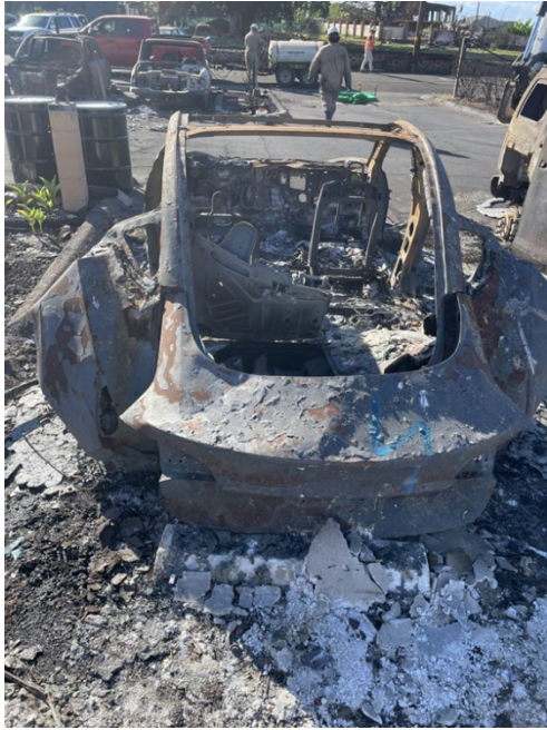
Figure 5: Tesla vehicle damaged by fire (left) and battery pack undercarriage with cylinder cells being harvested. While the battery pack may still be fully intact, the cells may be damaged and present a risk of thermal runaway and propagation.
