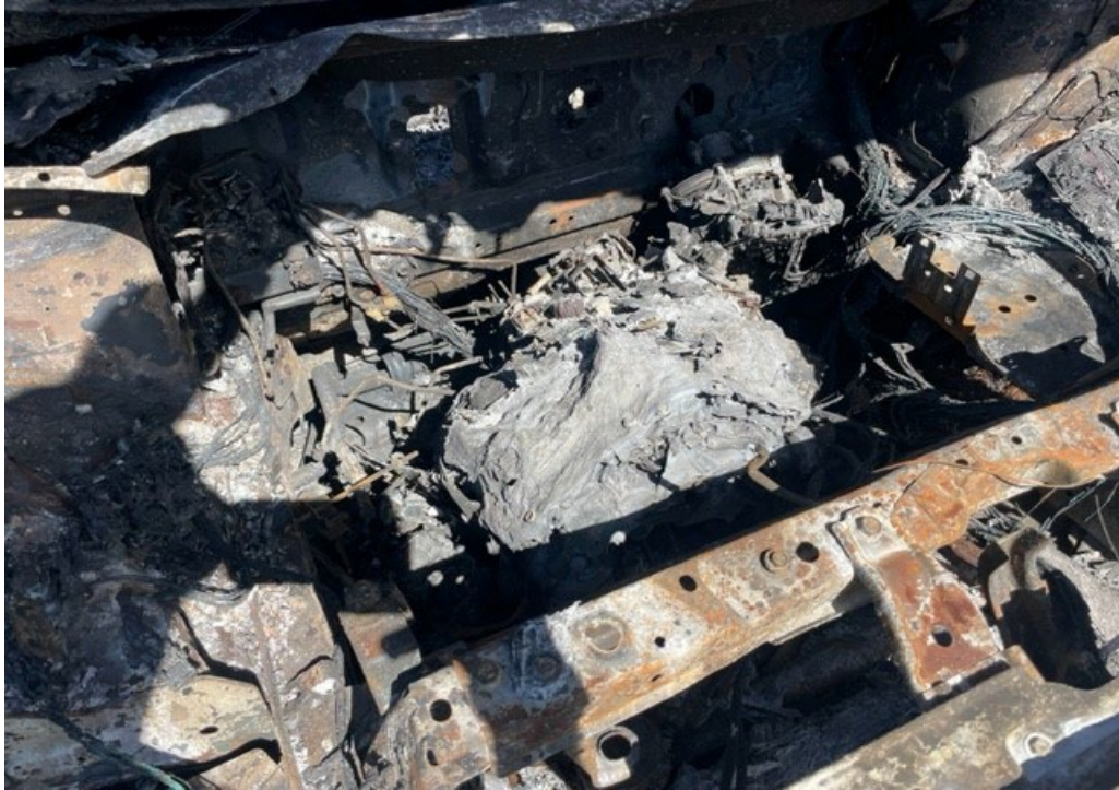
Nissan Leaf full electric vehicle engine bay. Note none of the components of a gasoline engine can be distinguished.
