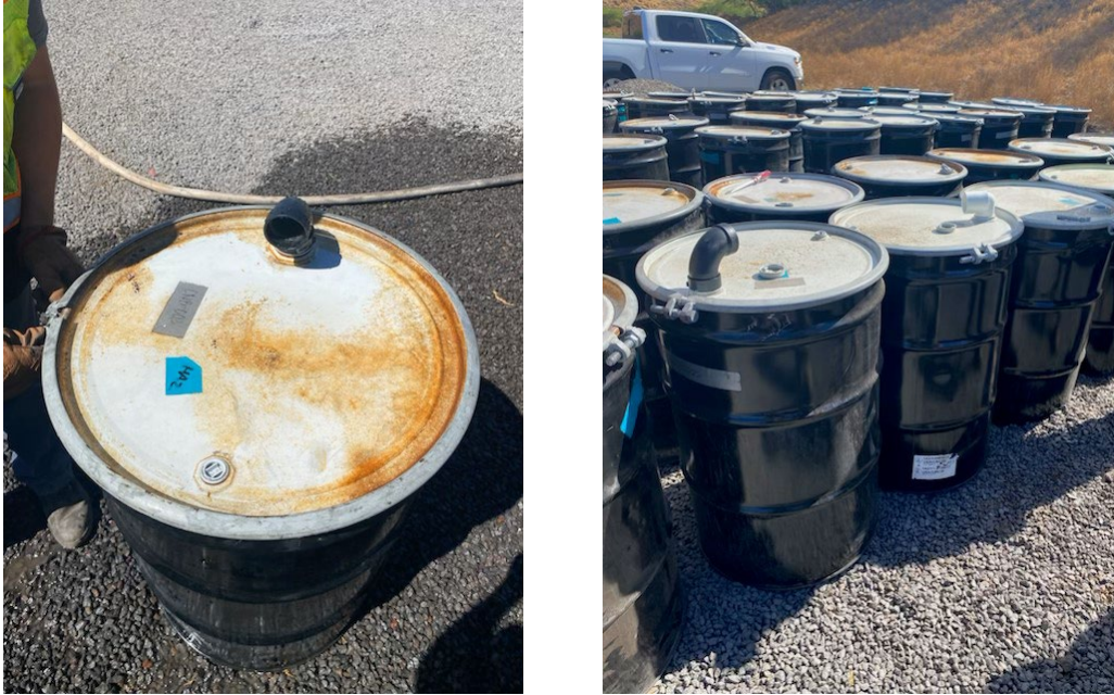
Figure 16: Using 55-gallon drums equipped with a ventilation snorkel can be used to safely store and transport material.
