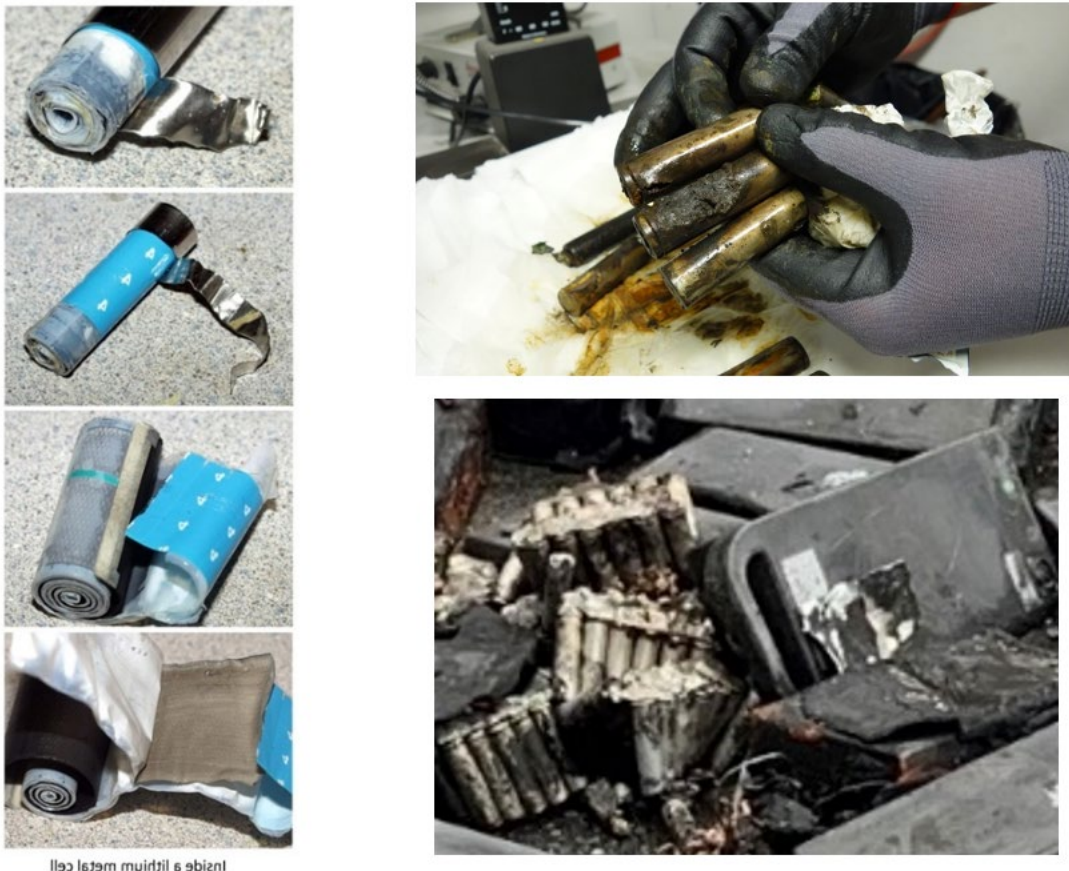
Figure 4: (Left) Lithium metal battery cell (not a lithium-ion battery) depicting a rolled-up strip of lithium metal; (Upper right) burned 18650 cells; (bottom right) fire-damaged cylindrical cells.
