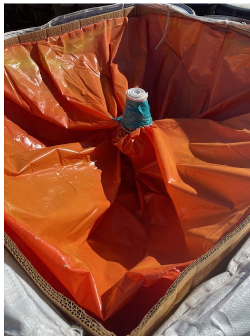
Figure 15: Cubic yard boxes with liners inserted into a supersack. A sorbent pad is tightly rolled and inserted in the middle of the box to provide for ventilation and protection from water intrusion.
