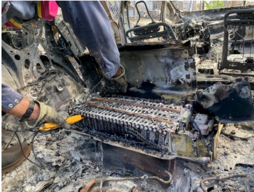
Certified electrician testing Ni-MH battery pack for remaining battery charge prior to removal
