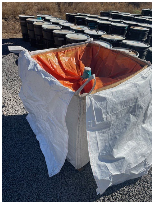
Figure 15: Cubic yard boxes with liners inserted into a supersack. A sorbent pad is tightly rolled and inserted in the middle of the box to provide for ventilation and protection from water intrusion.
