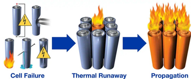
Figure 1: Diagram depicting a cascading thermal runaway event.
