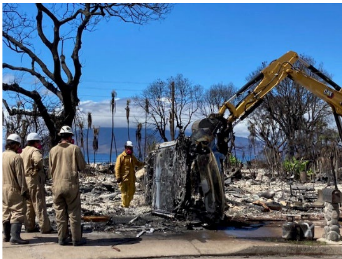
Flipping Tesla Model S to access batteries in undercarriage.
