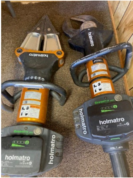
(Left) Rescue spreader and cutter. (Right) Cutting roofing support beams (A, B, C pillars) prior to flipping vehicle for battery pack access on some vehicles.
