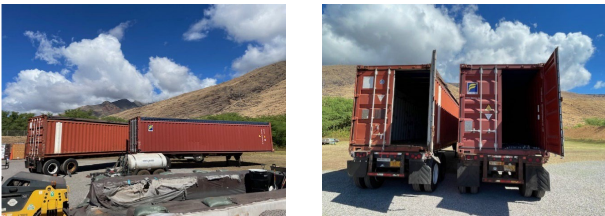
Figure 17: Transport containers that are open top with tarps. These should be placed above-deck when using barge or ship services.
