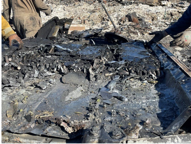
Figure 5: Tesla vehicle damaged by fire (left) and battery pack undercarriage with cylinder cells being harvested. While the battery pack may still be fully intact, the cells may be damaged and present a risk of thermal runaway and propagation.
