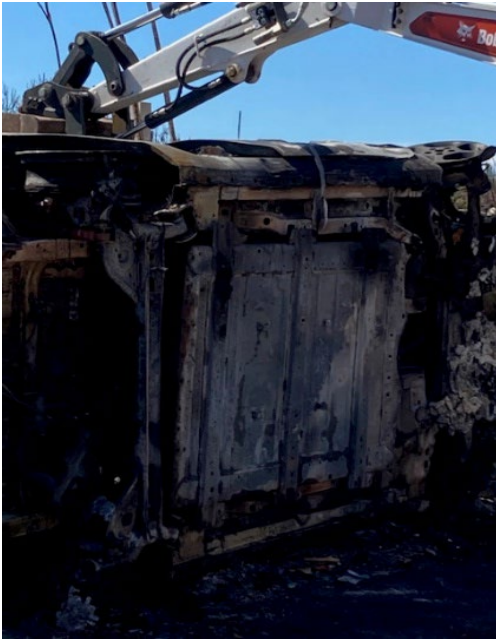
(Left) Nissan Leaf li-ion battery pack in undercarriage. (Right) Nissan Leaf battery pack after removal.
