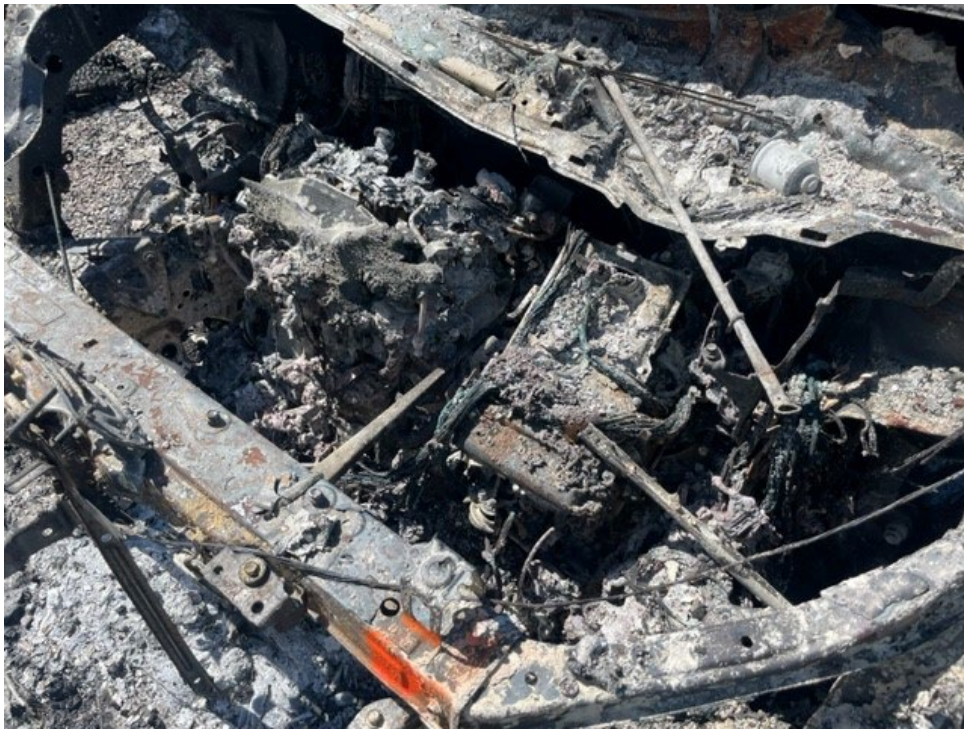
Toyota Sienna hybrid engine bay. Note electric motor components above transaxle coupled with typical 4-cylinder gasoline engine.
