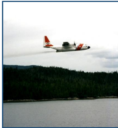
Test of aircraft dispersant application equipment during CANUSDIX drill. (ADEC Photo)
