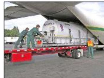
An Airborne Dispersant Delivery System (ADDS) unit is loaded into a cargo plane during a drill.
