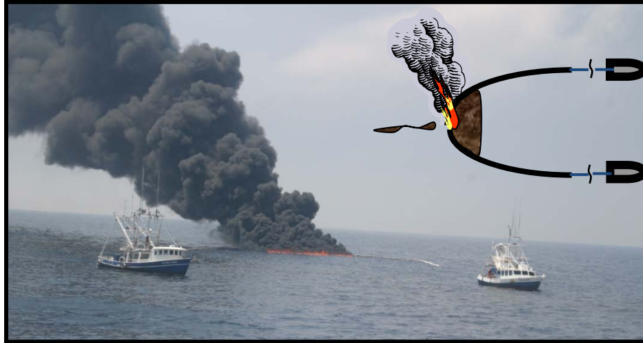
Figure 9407-6: Boats pulling fire boom in a U-configuration (DWH Spill – 2010)
