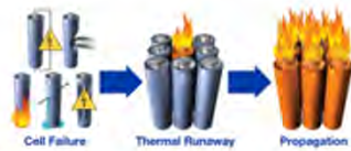
Figure 1: Diagram depicting a cascading thermal runaway event.
