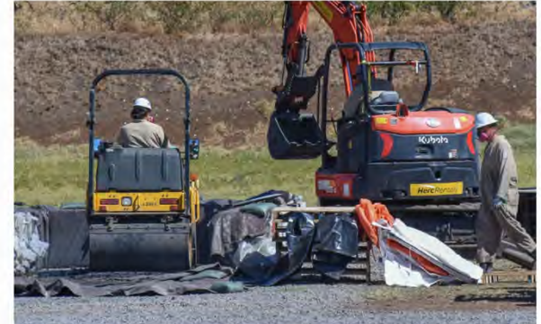
Workers at an EPA temporary processing site in Olowalu use a drumroller to crush lithium-ion batteries from the Lahaina burn site before they are shipped to the mainland for recycling of rare metals and disposal of what's left. PC: Cammy Clark
