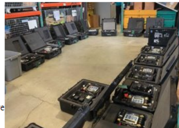
(Left) PO2 Josh Rice set-up AreaRae and ProRae Guardian with EPA ERT and EPA Region I START Contractor
