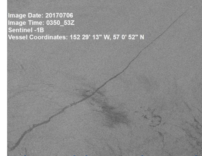
Widening with distance and connected to a vessel; possible illegal discharge
